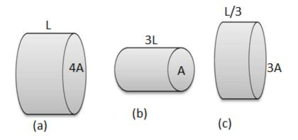
Solution. The relationship between resistance, length, and crossectional area of a conductor is following
