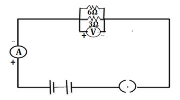
Solution.Let the current flows through  $3\Omega$  resistor is  $I_1$  and through  $6 \Omega$  resistor is  $I_2$  and current flow through the cell is I
